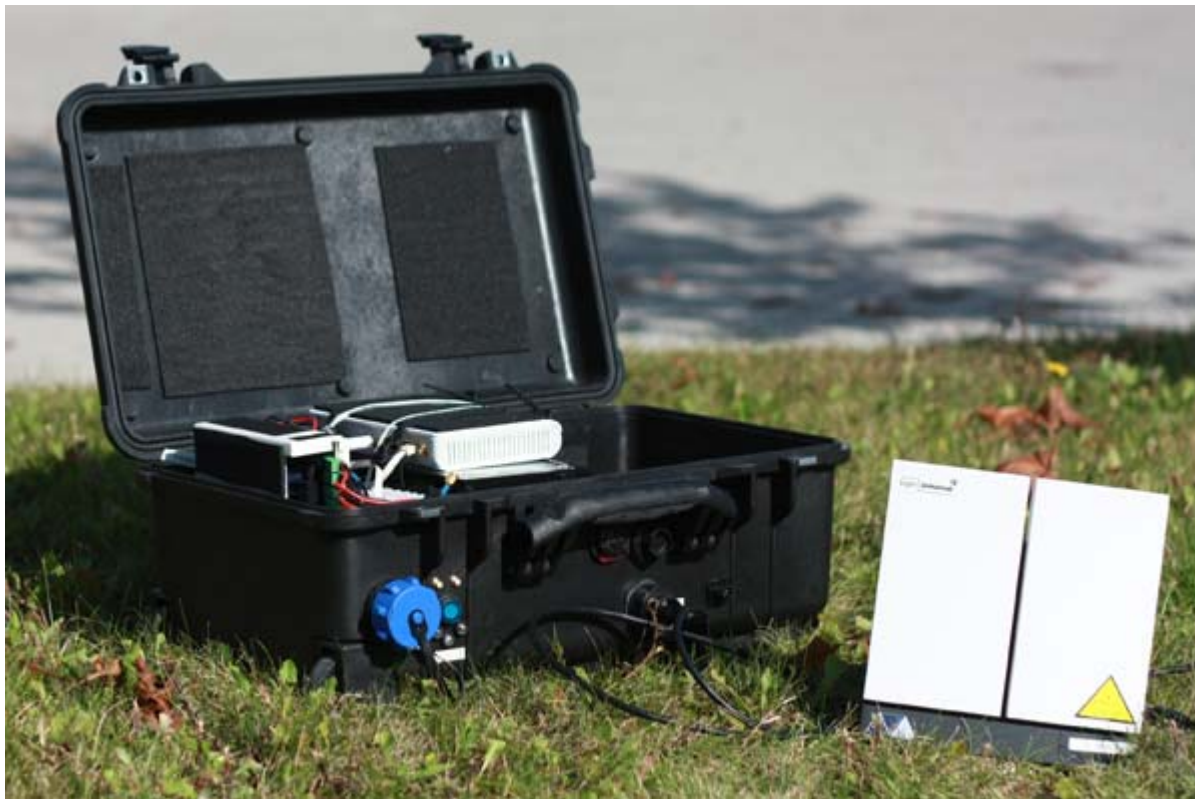
Figure 3: e-Triage communication suitcase (on-site emergency communications equipment, OSECE) consisting of an Inmarsat BGAN satellite terminal, a GSM pico cell, and a WLAN router (9).
