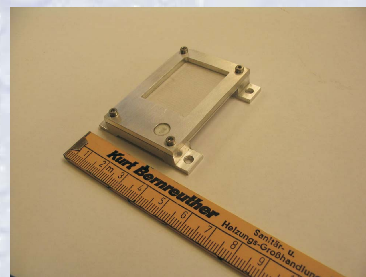
Fig. 7: First Breadboardmodel of HUM. The coulometric and capacitive sensor placed inside a small sensor housing (55 x 48 x 9 mm 3 )
