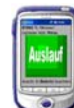
ENaflex-S works on a PDA and shows when to coast or brake
