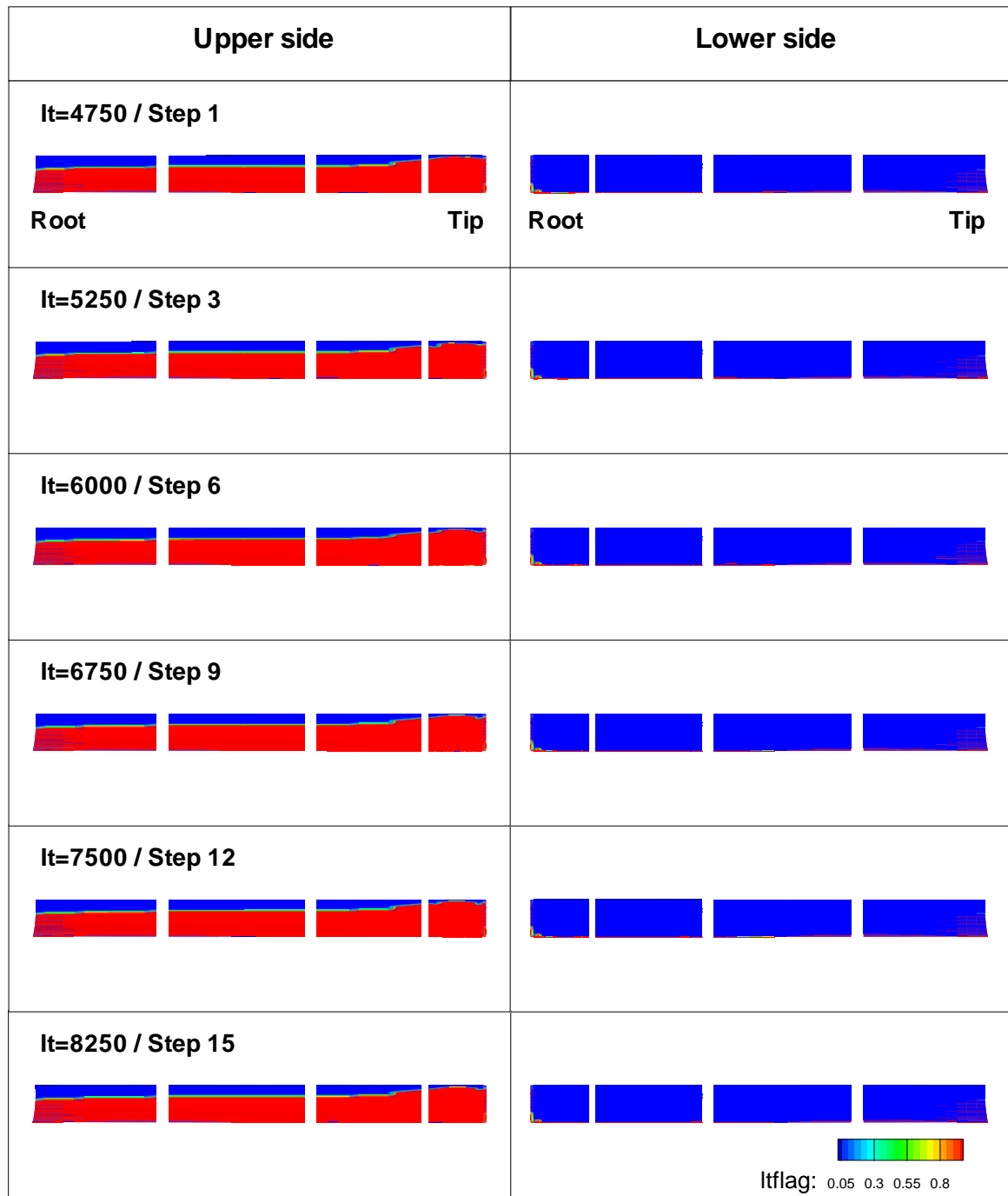
Figure C.11: ONERA 7A rotor - development of laminar and turbulent flow regions between selected transition prediction steps using the Michel criterion (version 1952 [19]).
