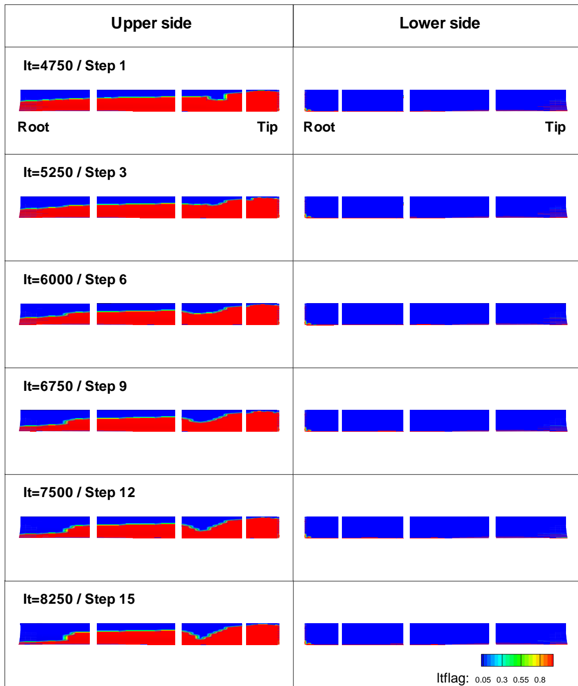
Figure C.7: ONERA 7A rotor - development of laminar and turbulent flow regions between selected transition prediction steps using the Michel criterion.
