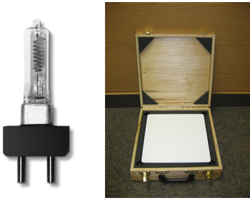
Figure 2: Tungsten-halogen lamp (left) and reflectance panel (right).
