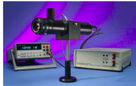
Figure 7: Components of a filter radiometer [7]. The CHB radiometers have a baffle tube instead of a lens.
