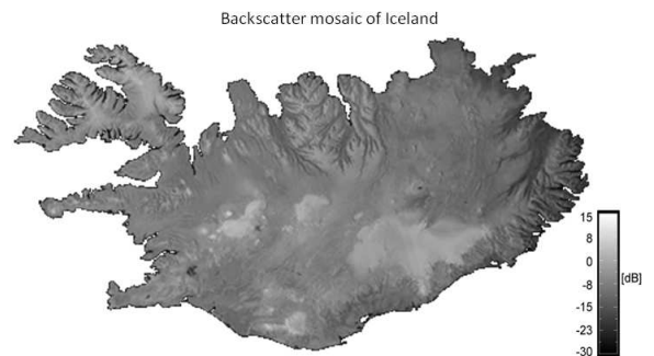
Fig. 8. X-Band global backscatter map (mean value) for HH polarization, after filling gaps of missing data.
