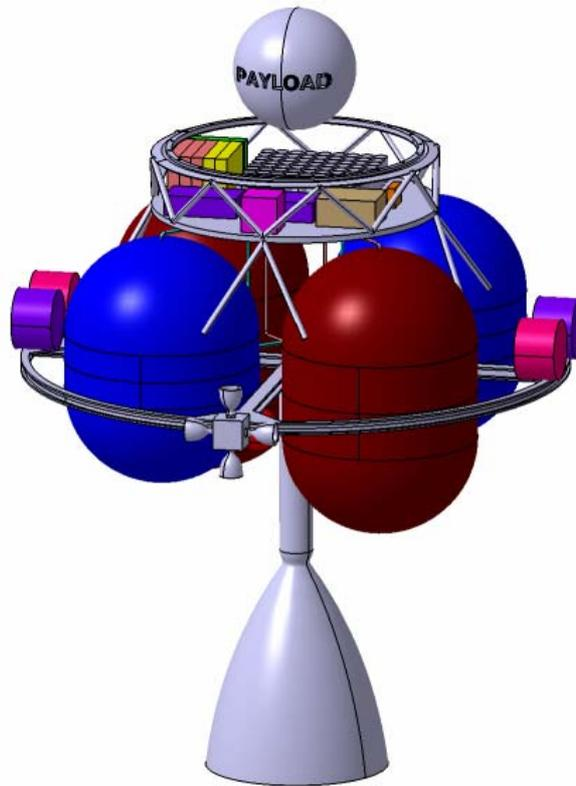
**Figure 5: Final design of kick-stage at the end of phase 0 study [6]**
