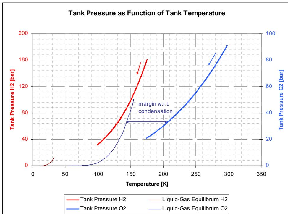
**Figure 4: Tank pressure as a function of temperature for O2 and H2 in pressure fed kick-stage [6]**
