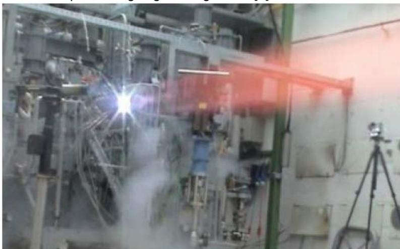
**Figure 3: Hot run #2 at P8 (December 2008) with approximately 9 MPa chamber pressure**
