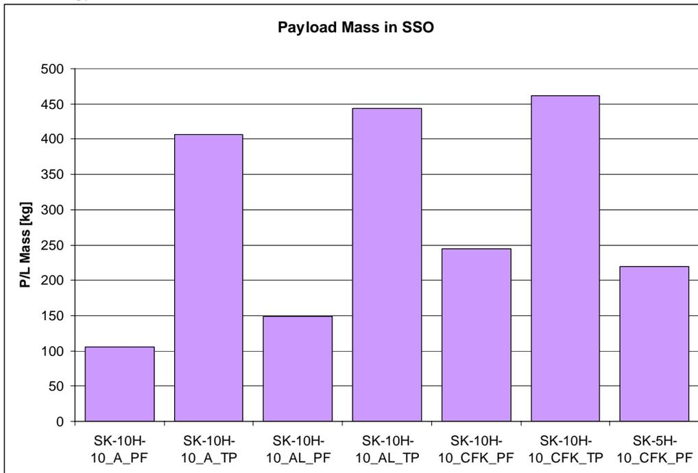
**Figure 7: Achievable payload mass with different engines and upper stage architectures of micro-launcher, PF: pressure fed, TP: turbopump fed, tank materials A: aluminium, AL: aluminium-lithium, CFK: filament wound CFRP) [5]**
