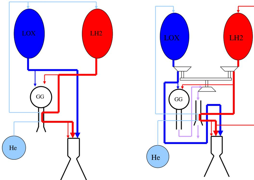
**Figure 6: Cycle options of small cryogenic upper stage with fully ceramic thrust chamber (left: pressure fed, right: turbopump fed) [5]**
