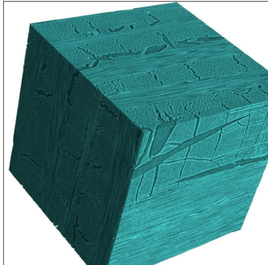
**Figure 2: Microstructure of C/C material**
