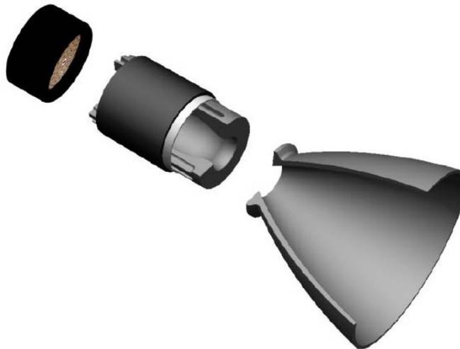
**Figure 1: Entire thrust chamber assembly in CMC as foreseen to be testfired**
