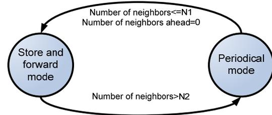
Fig. 4: Two mode model and switching mode conditions
