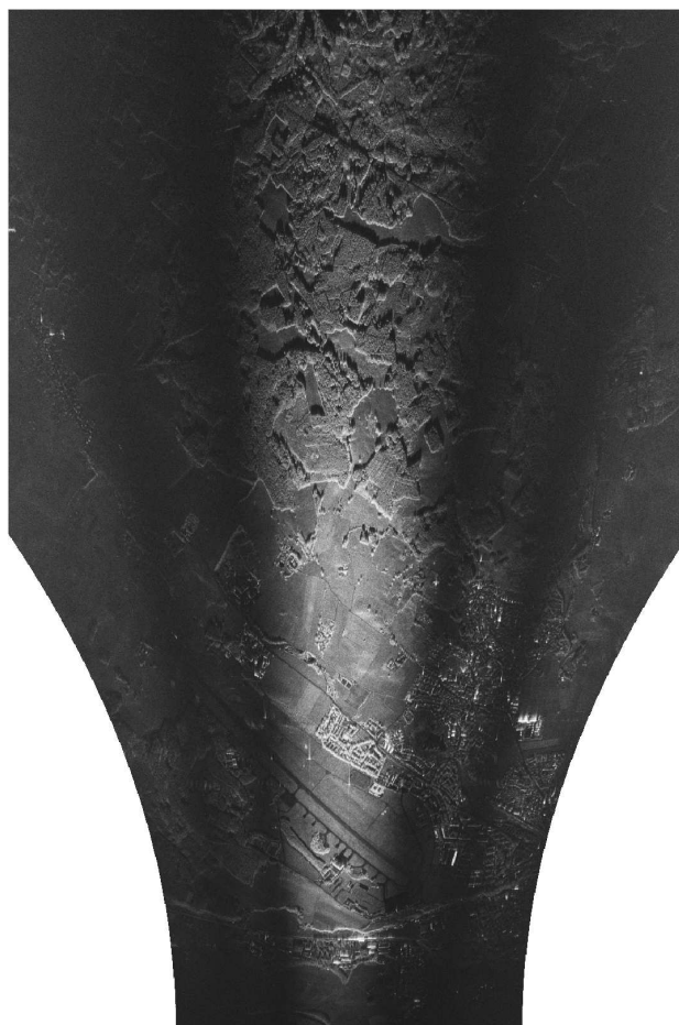
Figure 6: BFFBP-processed bistatic image of the TerraSAR-X/F-SAR first spaceborne-airborne experiment. Radar illumination from the bottom.
