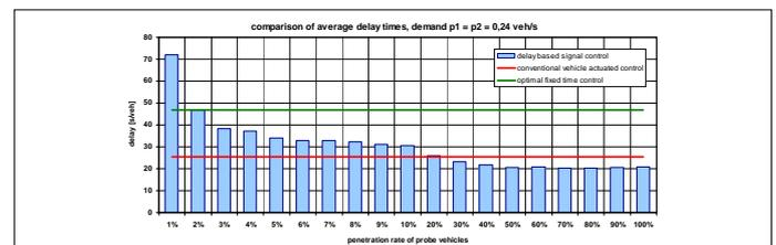
Fig. 3: Comparison of average delay times as function of the equipment rate of probe vehicles
