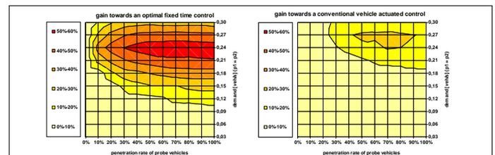
Fig. 2: Gain in travel time of the delay based control towards an optimal fixed time control, based on the Webster equation, and a conventional adaptive control, actuated by time gaps
