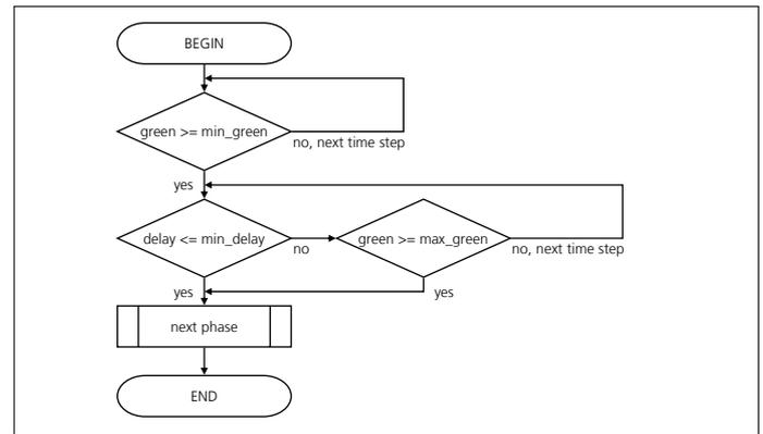
Fig. 1: Controlling scheme for one phase of the delay based signal control
