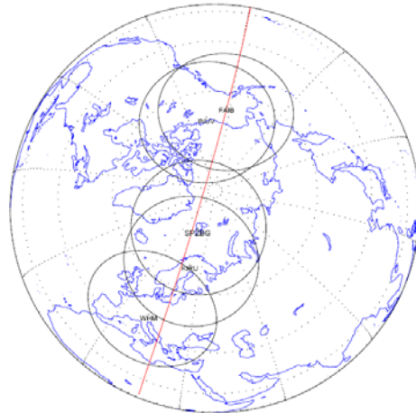
Figure 3: Chain of ground stations to extend contact times in low earth orbit (DEOS)
