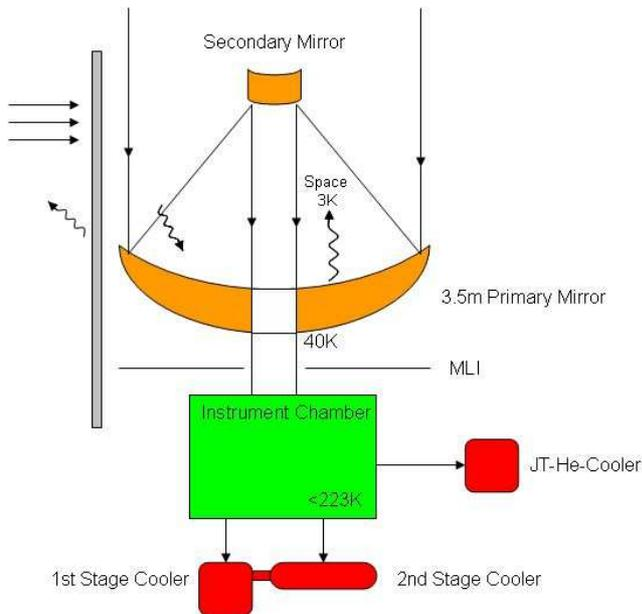
Figure 6: Telescope configuration
