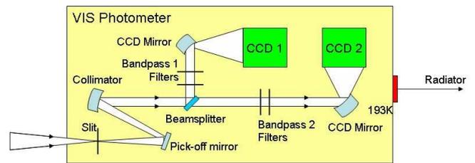
Figure 8: Photometer schematics
