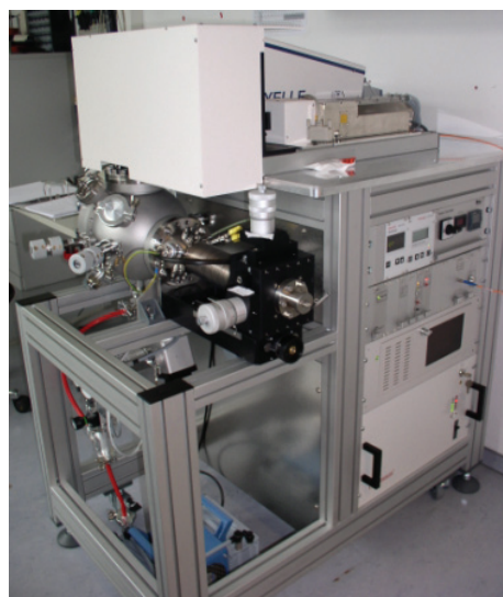
Figure 1: LIBS system with planetary simulation chamber.
