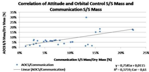
Figure 14: Correlation of attitude and orbital control S/S and communication S/S of exploration systems (1958 to 2010)
