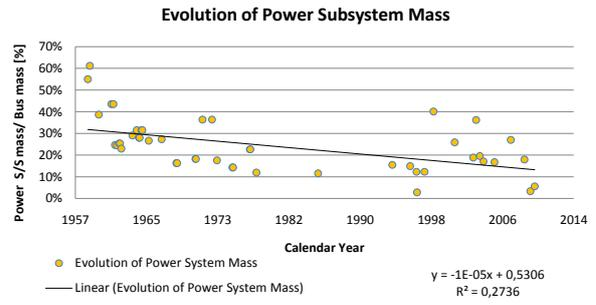
Figure 10: Evolution of power subsystem mass of exploration systems from 1958 to 2010
