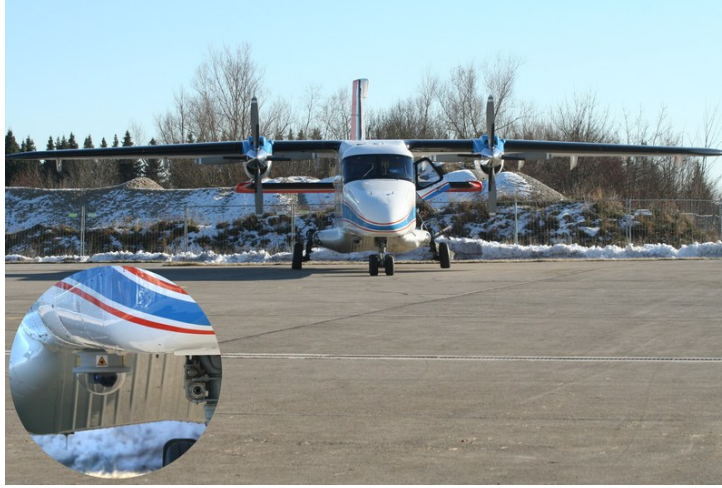
Figure 1: Picture of the Do228 Aircraft with Installed Optical Terminal. Lower Left: Enlargement of Coarse Pointing Assembly
