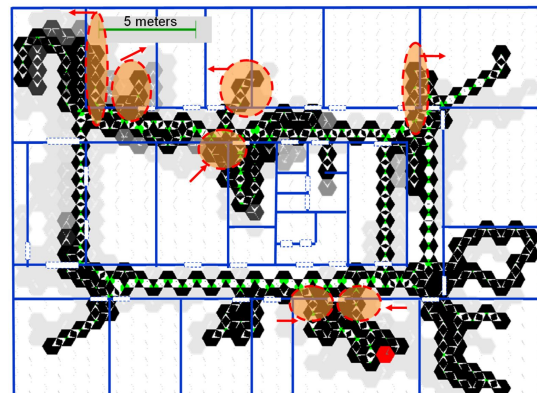
Figure 2. A map learnt from foot mounted IMU data alone plotted on the actual building layout for reference. See Figure 4 for explanations.
