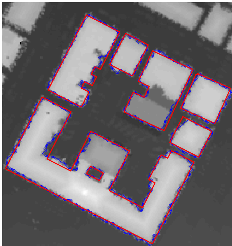
Figure 7.15: Building outline approximation result ( red polygons ) as well as the original extracted building boundaries ( blue polygons ) superimposed on LP image
