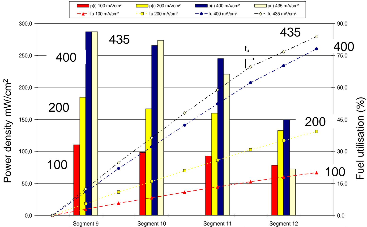
Anode supported cell, LSCF cathode, 73,96 cm<sup>2</sup>, gas concentrations (current density equivalent): 54.9% N<sub>2</sub>, 16.7% H<sub>2</sub>, 16.5% CO, 6,6% CH<sub>4</sub>, 2.2% CO<sub>2</sub>, 3.2% H<sub>2</sub>O (0.552 A/cm<sup>2</sup>), 0.02 SlpM/cm<sup>2</sup> air
