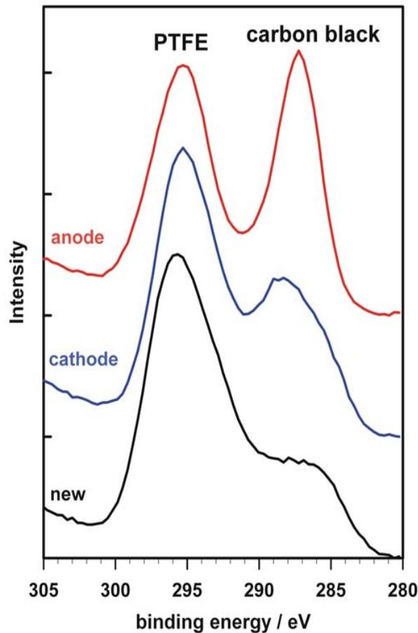
➤ Partial decomposition of PTFE identified by X-ray photoelectron spectroscopy
