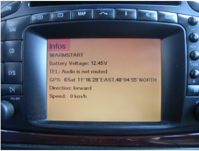
Figure 3: Debug Information System: The debug information system of the Mercedes G400 delivers battery and audio status, the coordinates as measured by the in-vehicle navigation unit, the driving direction as set by the automatic gear and the current speed as measured by the odometry.
