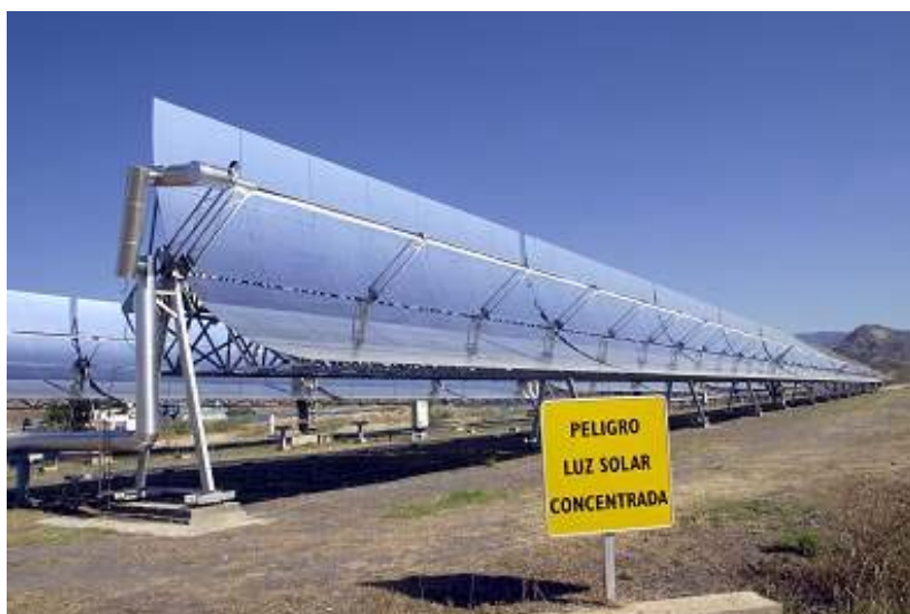
Figure 3-39: View of the two ET-100 collectors installed at the DISS test facility in 2003 (PSA)
