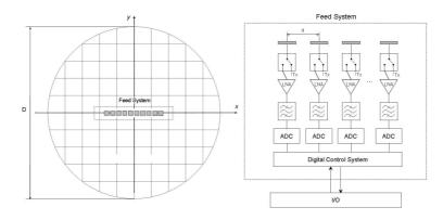
Fig. 1. Simplified architecture of the reflector based DBF SAR system: the reflector dish with a schematically depicted feed system (left) and a simplified structure of the digital feed system circuitry (right).
