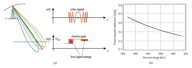
Fig. 2. a) Pulse extension loss principle. b) Angular pulse extension on ground as a function of ground range.
