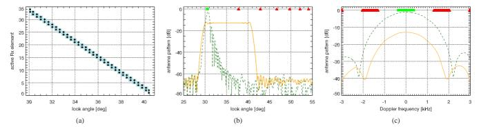
Fig. 3. a) Feed activation matrix as a function of a look angle. b) and c) Elevation and azimuth antenna patterns correspondingly (solid line - Tx, dashed line - Rx).
