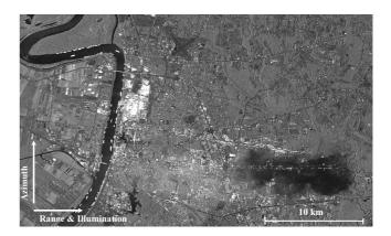
**Fig. 1**. An example of a SAR image with rain-cell signatures recorded with TerraSAR–X in the US close to Baton Rouge. The white shading is due to direct reflections from the rain region (shown as volume 'A' in Fig. 2). Whereas the darkly shaded areas are due to rain attenuated (blocked) signals from the ground; this effect is shown as region 'B' in Fig. 2.
