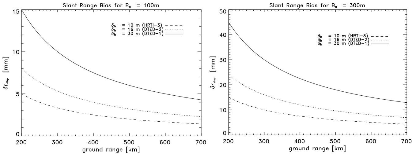
**Figure 4** Plots of the absolute LOS deformation error (in slant range) across the RCM accessible ground range swath for different DEM (type) bias considering a baseline of 100 m and 300 m, respectively.
