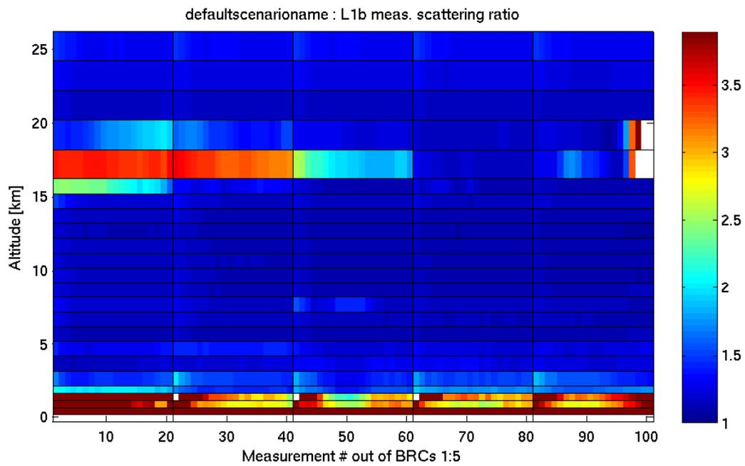
**Figure 2.** Scattering ratio for Aeolus simulations based on LITE-period data. Upper panel: E2S input (high resolution truth), lower panel: L1B retrieval at instrument measurement resolution.
