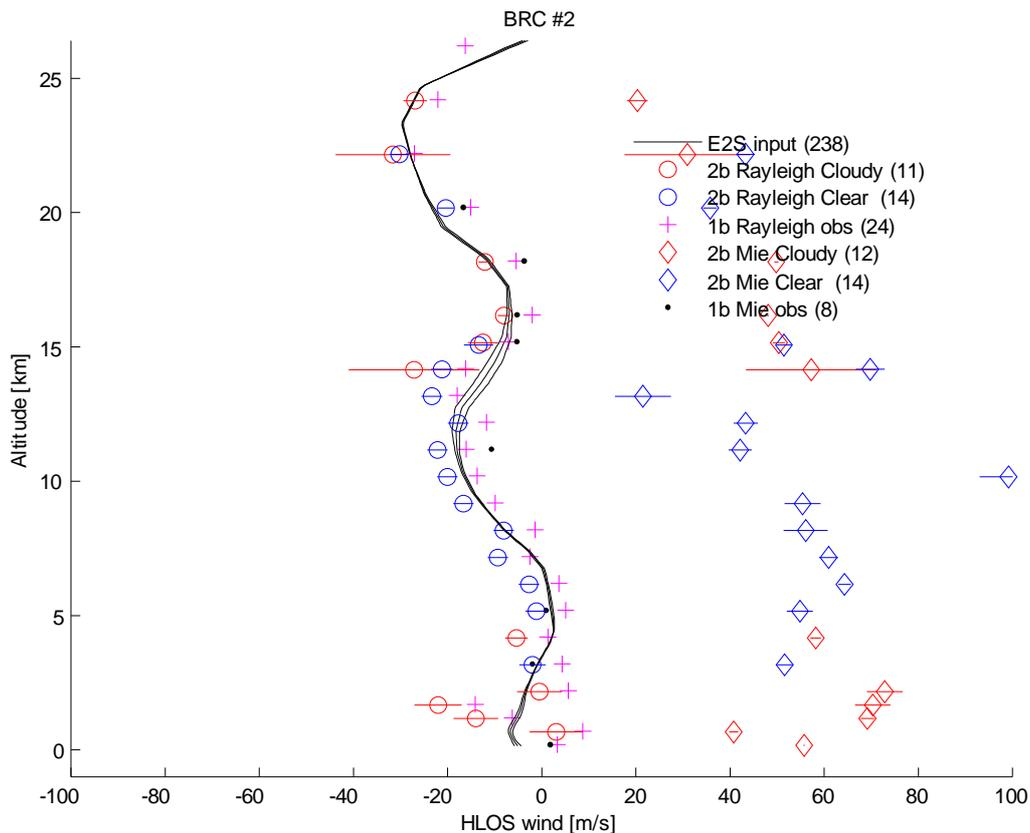
**Figure 3. True wind profile (E2S input) and simulated retrievals (see legend). The large offset of the L2B Mie retrievals (diamonds) has been traced to a systematic error in the L1B data used as input to the L2B processor.**
