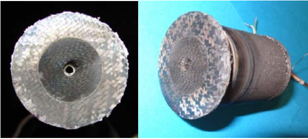
Figure 20: RESPECT [023084L] after testing – T_{\max}=2500^{\circ}\text{C} .
