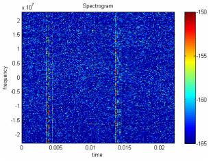
Figure 20: Spectrogram of recording "HM E5a 13" showing two occurrences of pulsed interference.
