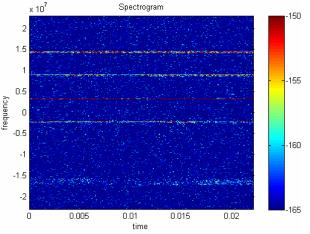
Figure 9: Spectrogram of dataset "MH E5a 173" showing several narrowband interferences and one broadband interference at roughly -1.5 MHz. Power density in dB(mW/Hz). Frequency from bottom to top represents the frequency relative to the middle frequency. Time from left to right represents the time into the recording in seconds.
