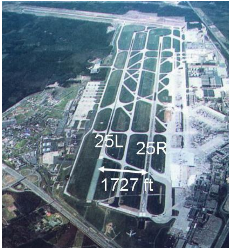
Fig. 1. Frankfurt Airport with the two parallel runways 25L and 25R, spaced by 1727 feet (518 m).
