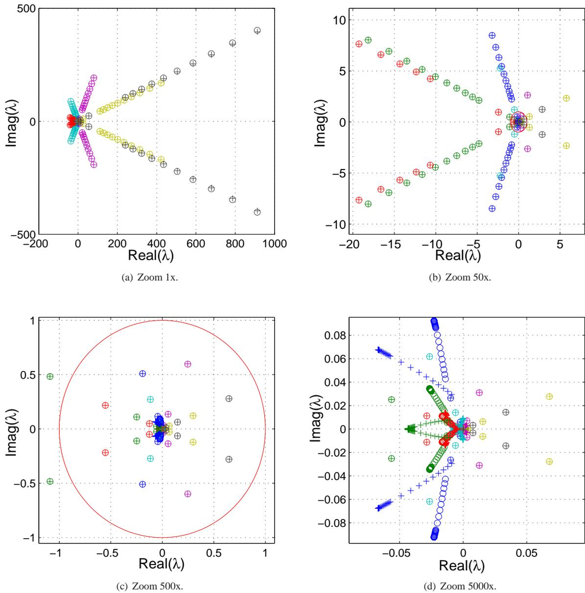
Fig. 3. Comparison of closed-loop characteristic multipliers: Floquet theory (o) vs Pole placement (+). In the special case of a momentum bias spacecraft, the approximate stability results obtained via the pole placement-based design technique proposed in [2] match very accurately with the exact ones derived in the framework of Floquet theory.
