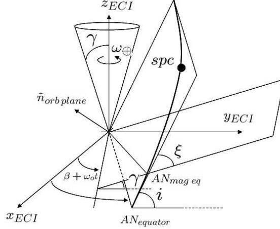
Fig. 2. The geomagnetic field tilted dipole model.
