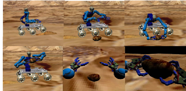
Figure 14. Rovonaut: Different scenes (taken from animation) for demonstrating surface exploration, sample collection and inspection
