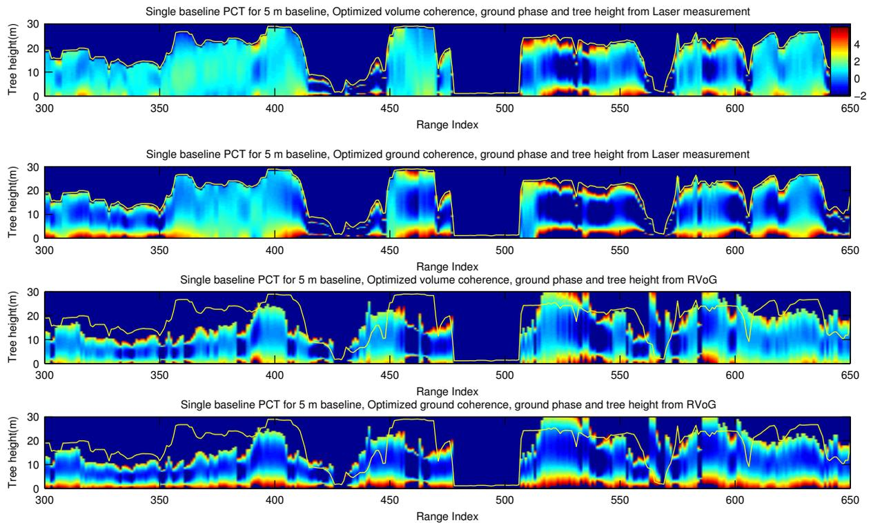
**Fig. 5.** Single baseline Polarimetric Coherence Tomograms (PCT) for L-band 5 m baseline optimal coherences with two different initial value sets. PCT in upper two panels are calculated by using laser measured DEM and tree height, lower two panels are calculated by using ground phase and tree height derived by RVoG model inversion. Yellow line represents laser measured tree height (m) in all panels. All the panels have same color scale.
