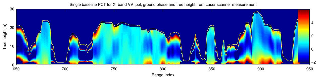
**Fig. 2.** Coherence tomogram profile for single baseline X-band VV polarization measurement. Ground phase and tree height are obtained from laser scanner measurement. On the x-axis is range index. Note the difference between mixed forest (near range index 760) and the sparse pain forest (near range index 900).
