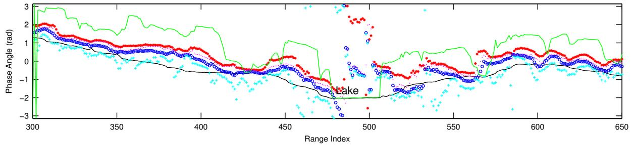
**Fig. 4.** Estimated ground phase  $\phi_0$  and coherence phases along the PCT track. The black line represents laser DEM generated ground phase, the red star and the blue circle are optimized coherence phases, the cyan plus stands for RVoG model estimated ground phase, the magenta dot shows HH+VV coherence, the green line marks treetop line in phase scale.
