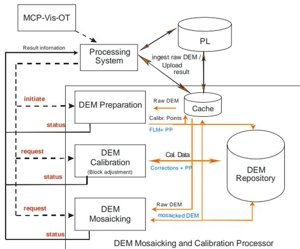
**Figure 2** Overview of the MCP components
