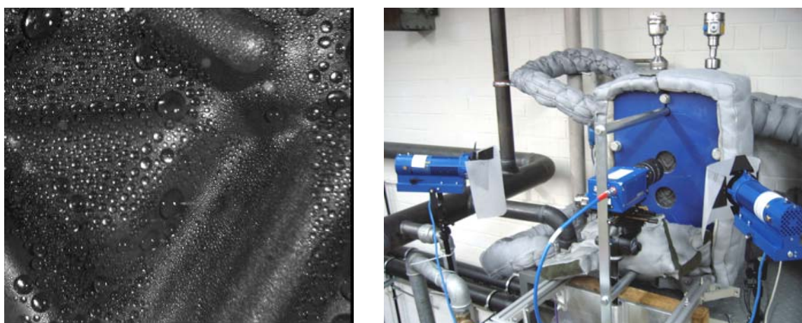
Figure 4: Left: Dropwise condensation on a coated heat exchanger plate Right: Test condenser with windows for visual observation and high-speed camera
