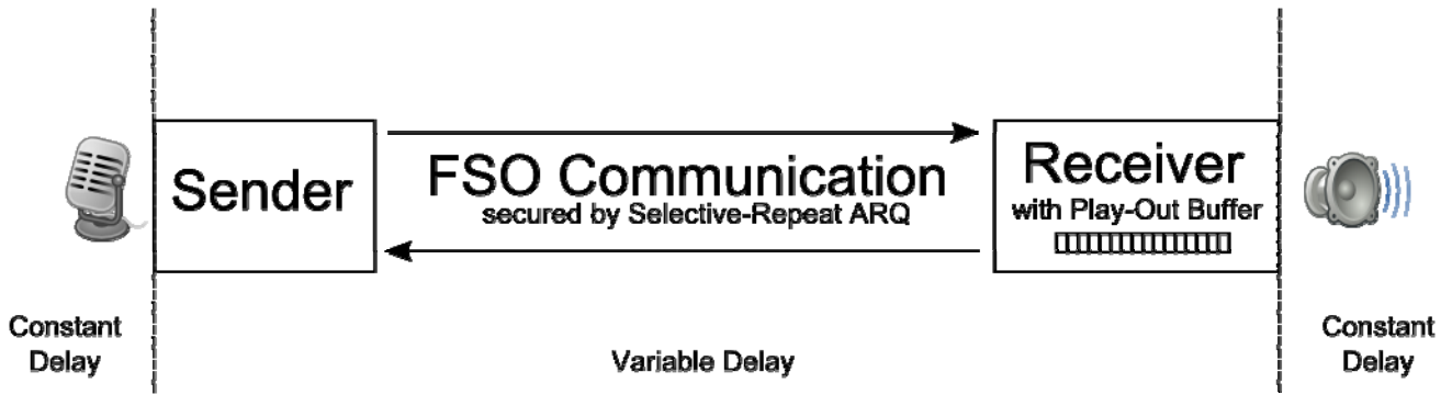
Fig. 3: Play-out buffer concept for removing variable delay introduced by ARQ protocol into the data flow.
