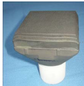
Fig. 2: Ceramic absorber module
