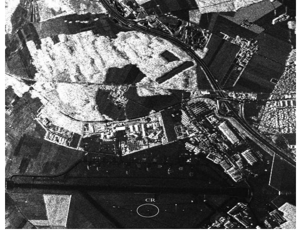
Fig. 4. Amplitude SAR Image (slave) at L-band used to demonstrate the WPCA algorithm. Range increases from left to right and azimuth from top to bottom.
