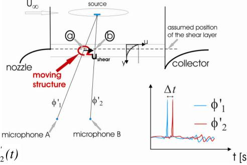
of a wave which propagates through a shear layer: velocity of structures
