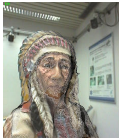
Fig. 9. Online triangulation with live camera stream augmentation.
