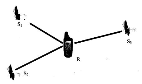
The velocity of light is a physical constant (approximately 300,000 kilometers per second); therefore the distance between the GPS receiver and the satellite can be calculated by measuring the time interval a signal takes to travel from the satellite to the receiver.
