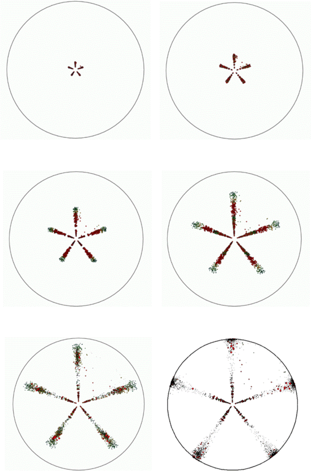
Fig. 9. Time-dependent spray formation emitting from a multi-hole nozzle.
