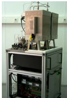
test setup for adsorbents for desulphurization
