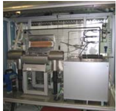
prereformer catalyst testing
