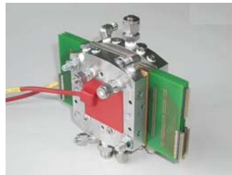
Fig. 2: Short-stack consisting of 3 cells with segmented bipolar plates
