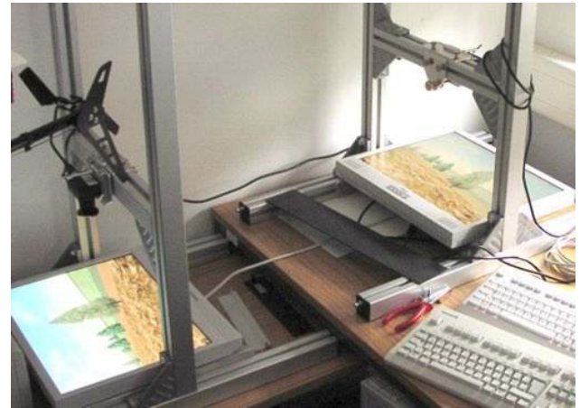
FIG. 12: Hardware-in-the-loop simulation by capturing images from displays showing generated views.
