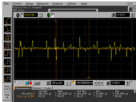
Figure B.1: Baseband DME/TACAN pulses generated by signal generator Agilent E8267D
