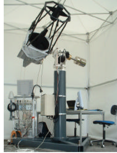
Fig. 2 Left: Optical terminal that flew on a stratospheric balloon in Capanina trial. The coarse pointing assembly is a periscope located on the bottom of the terminal. Right: Optical ground station used for Capanina trial.
