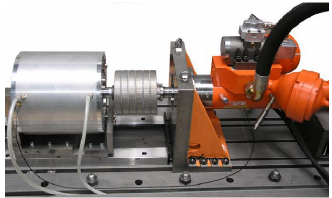
Fig. 2 Linear generator on the test stand
