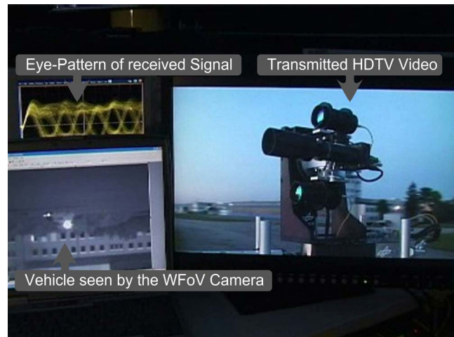
Fig. 3. Transmitted HDTV-Video from a moving van. The Van can be observed on the fixed terminal wide field of view (WFOV) camera. The transmitted video shows the mobile terminal optics. Also the current eye-pattern of the received signal is given [6].
