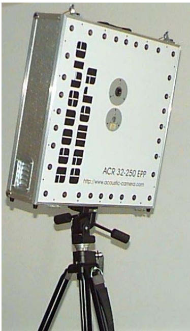
Fig. 1. Acoustic Camera: Combination of a microphone array with a video camera.
