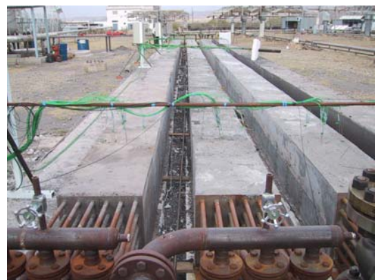
350 kWh concrete and cast ceramics test modules before mounting the thermal insulation
