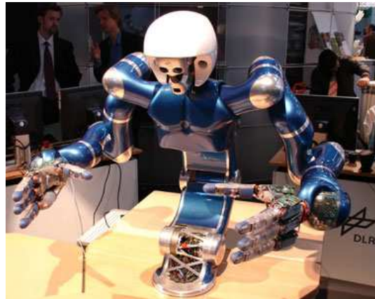
Fig. 1. An example for a complex robot system: the new DLR Two-Hand-Arm-Torso (THAT) with 43 DOF. This system is built from two DLR-LBR-III arms with 7 DOF each, two DLR-Hand-II with 13 DOF each [1] and a torso with 3 DOF.
