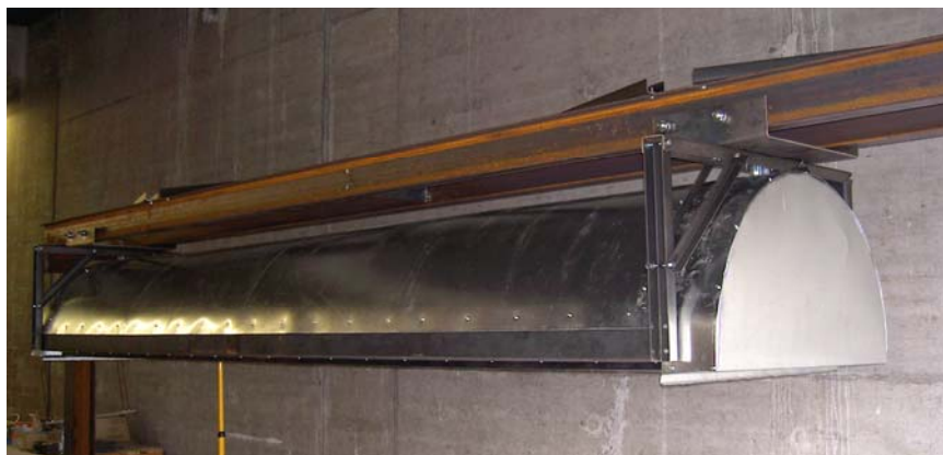
Figure 3: Receiver using a single tube absorber (4 m in length) installed by Solar Power Group
