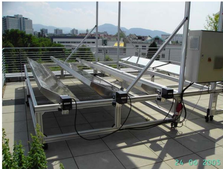
Figure 7: Test-stand for mirror tracking and control
